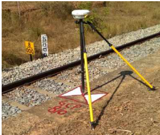
FIGURE 3.4: GCP OBSERVATION USING DGPS
