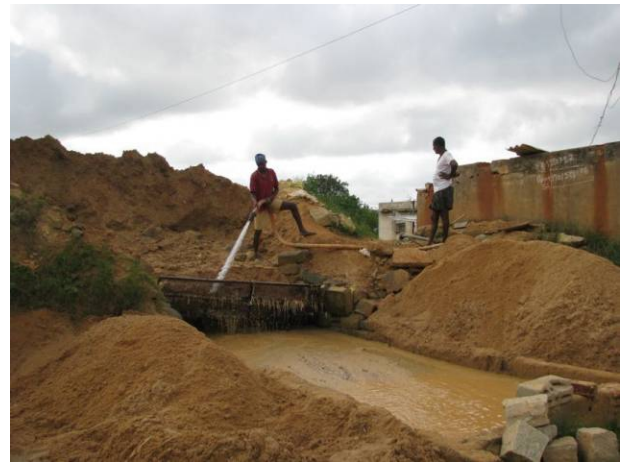
Picture 9b: Sand being segregated by jet stream processing with soil lifted from the lake bed.
