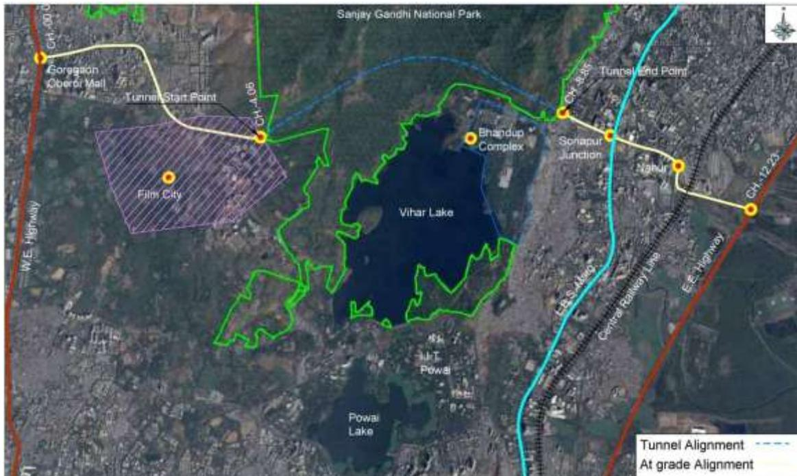
**Figure 7 GMLR Proposed Tunnel Alignment Option by M.s Padeco Co ltd**
