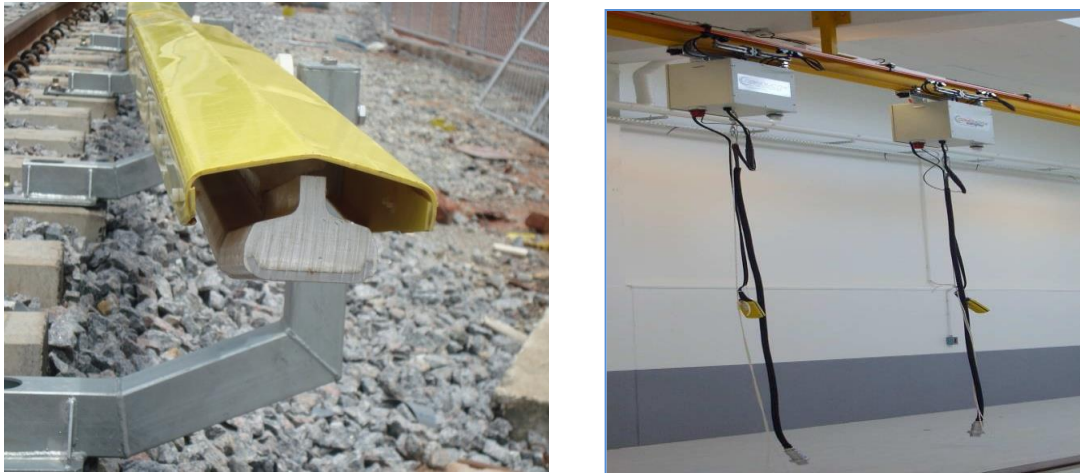
Figure 12.2 Third Rail and Stringer System
