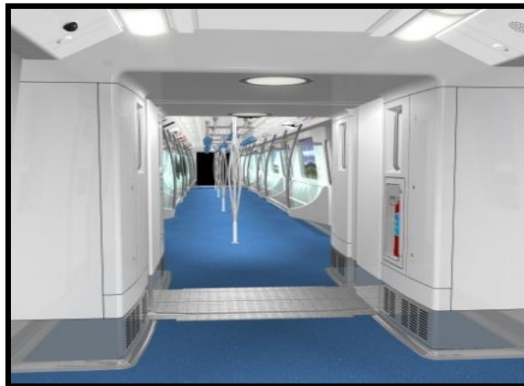
Figure 11.4 View of Gangway
