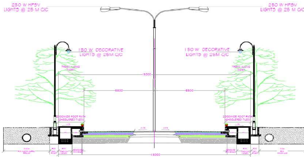
Cross Section of 15M. Wide Road
