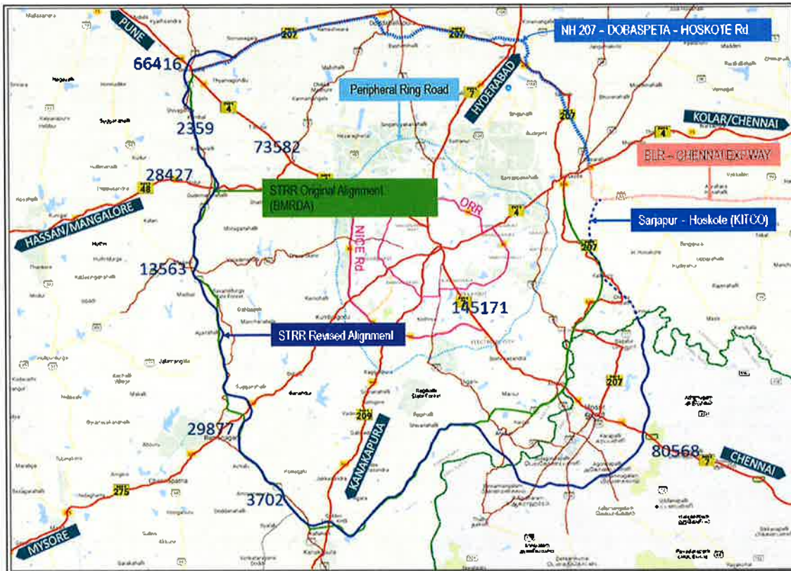
Figure 7.6 : Traffic Volume in PCU
