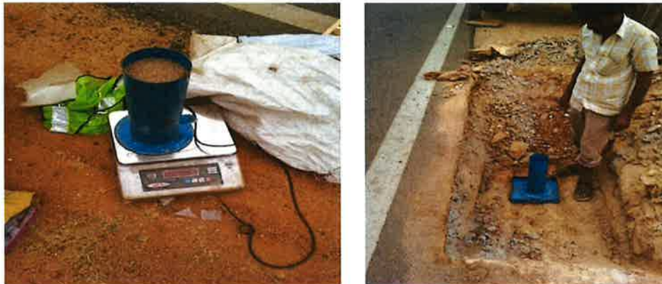
Figure 4-1: FDD and soil sample collection and DC testing at site
