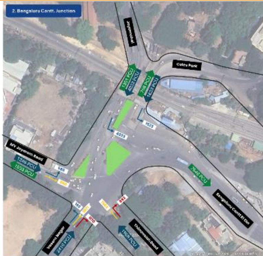
Figure 96: TMC at Bengaluru Cantt Junction
