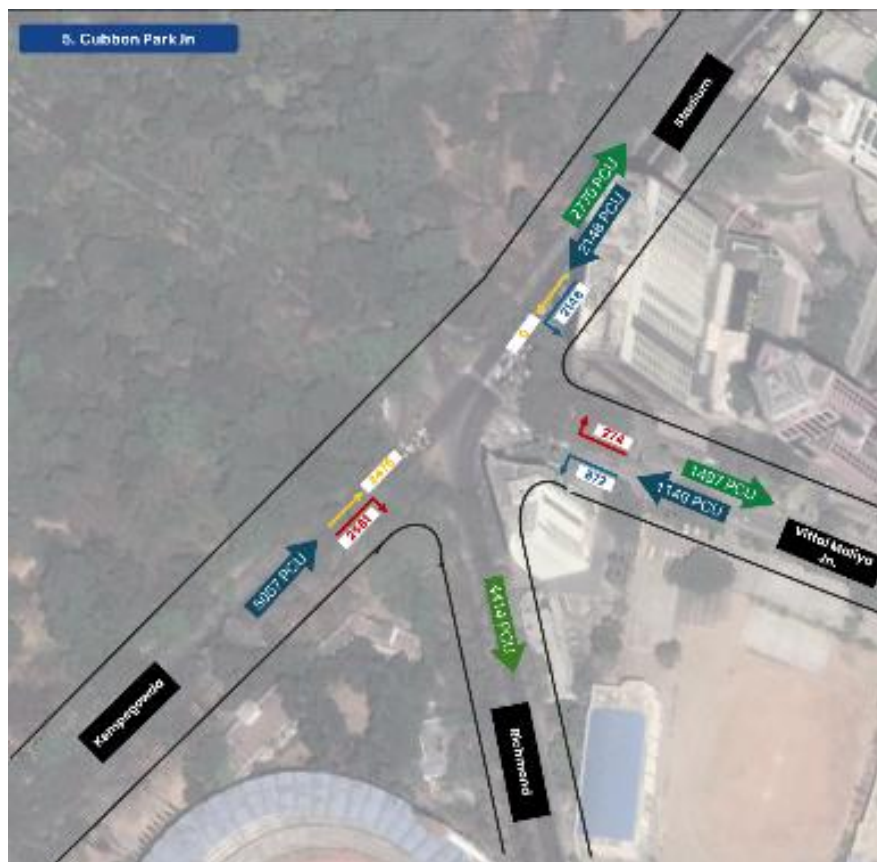
Figure 99: TMC at Cubbon Park Junction
