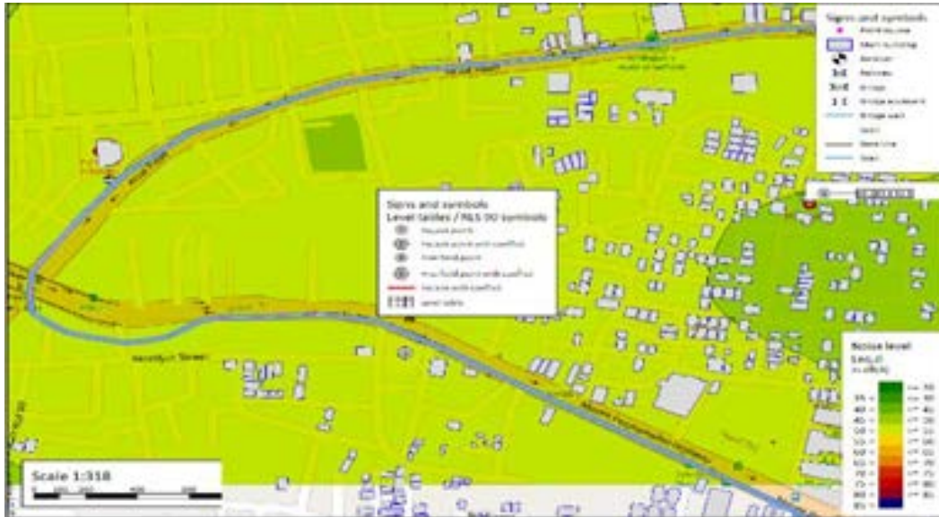
Figure 5-42: Poonamallee Government Hospital- Day time - Noise contour map for Operation phase after Mitigation
