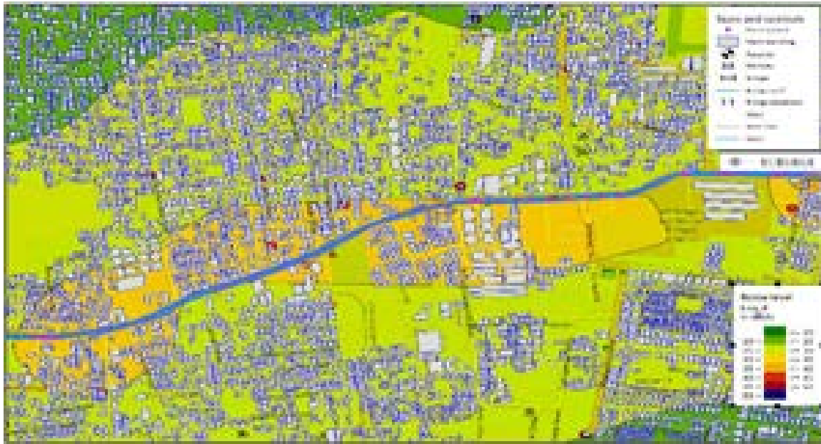
Figure 5-34: Narayanan E-Techno School- Day time - Noise contour map for Operation phase after Mitigation
