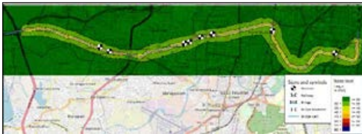
Figure 5-51: Operation Noise at overall – Night Time – With Mitigation Wall
