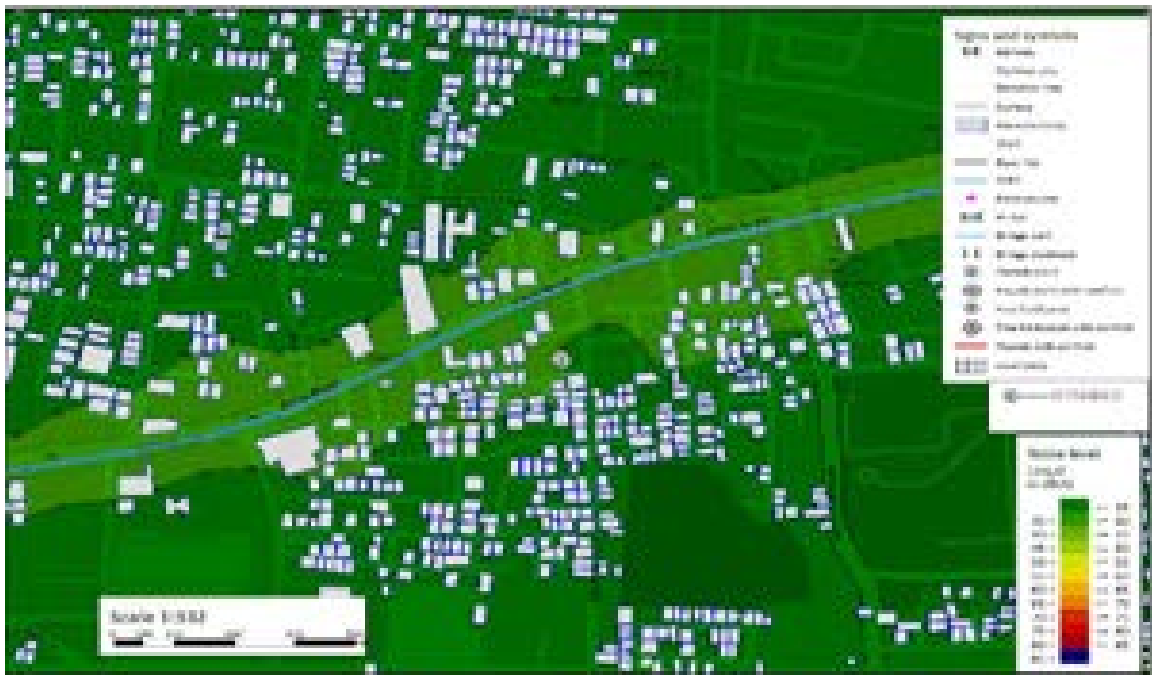
Figure 5-38: The Holy Cross Matric Hr.Sec.School- Day time - Noise contour map for Operation phase after Mitigation
