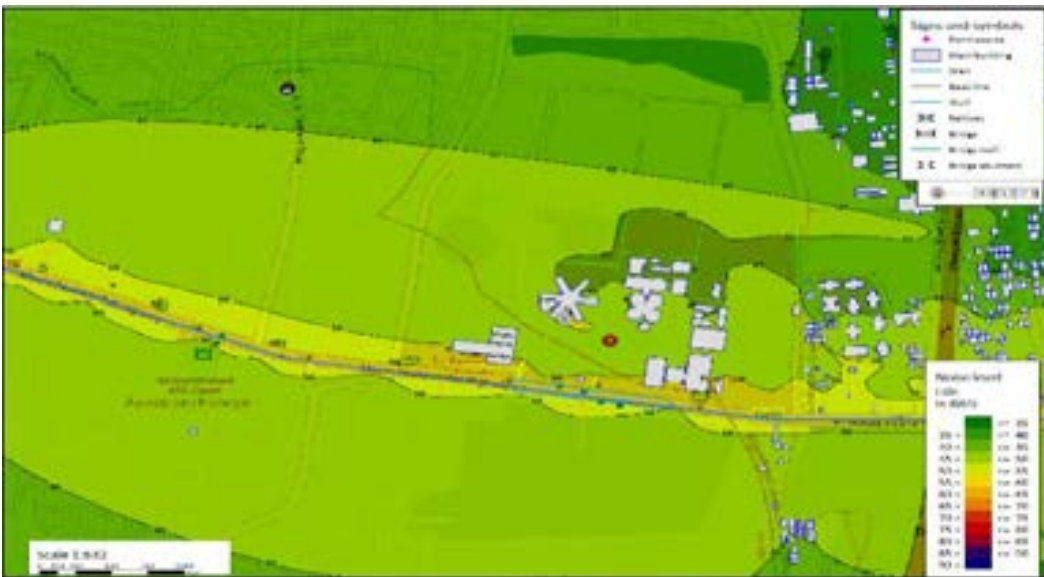
Figure 5-47: Sri Ramachandra Dental Hospital - Day time - Noise contour map for Operation phase after Mitigation
