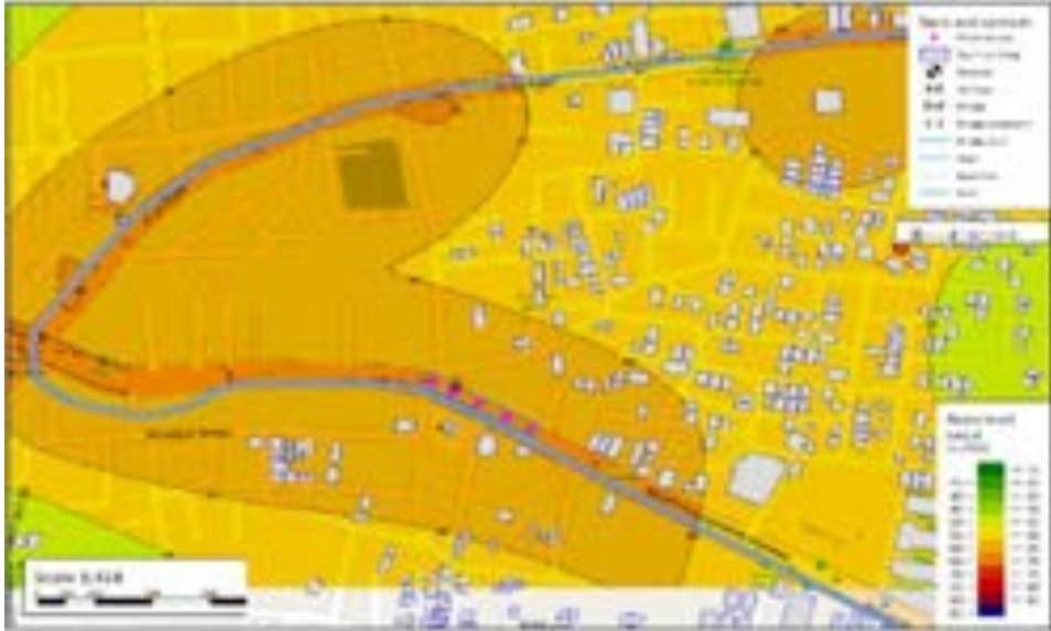
Figure 5-40: Day time Noise contour map for Operation phase (Mullai Thottam – Poonamallee Bus Terminus).
