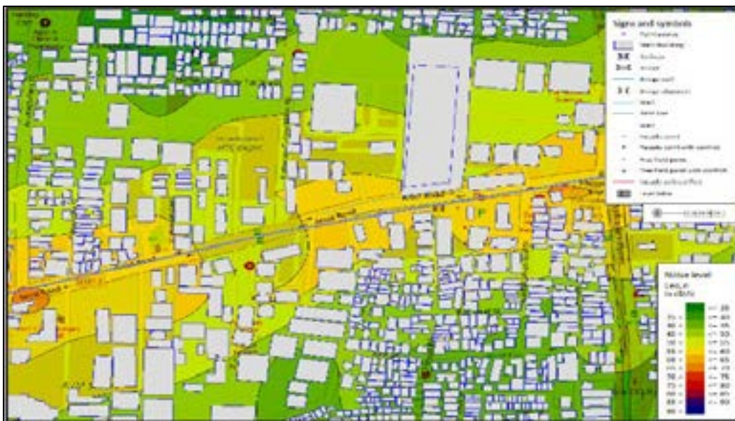
Figure 5-29: Night time Noise contour map for Operation phase (Vadapalani – Saligramam).
