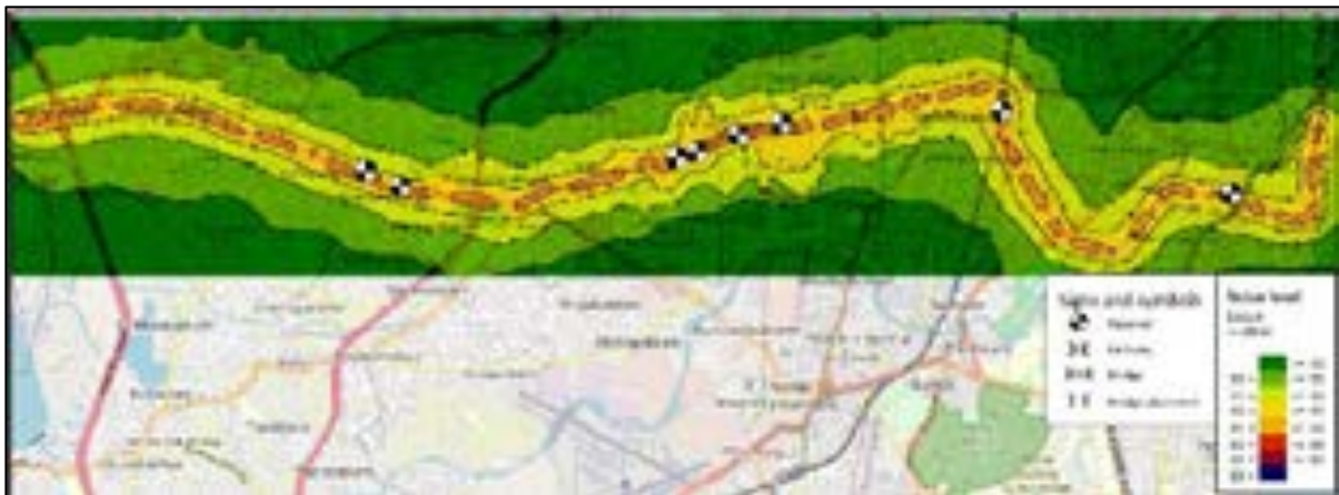
Figure 5-50: Operation Noise at overall - Day Time – With Mitigation Wall
