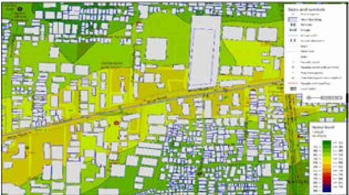
Figure 5-31: Vijaya Hospital- Night time - Noise contour map for Operation phase after Mitigation
