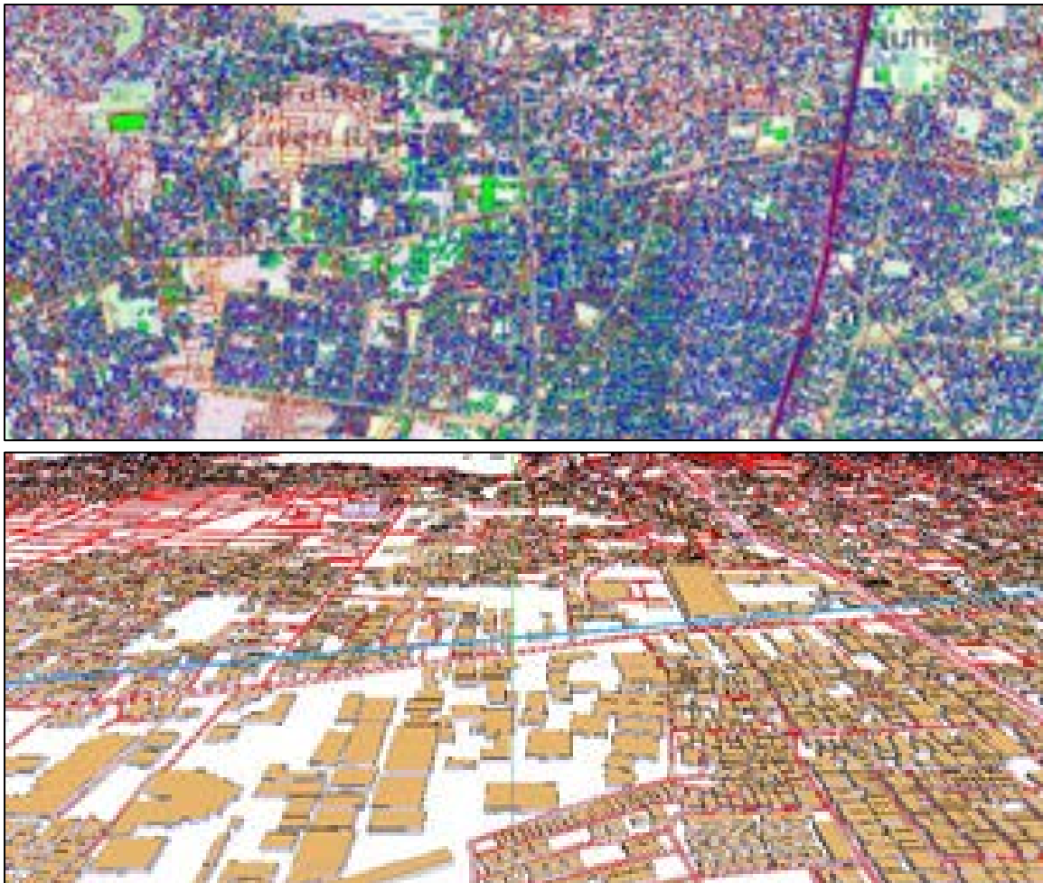
Figure 5-27: Sound Plan with input of buildings and Roads
