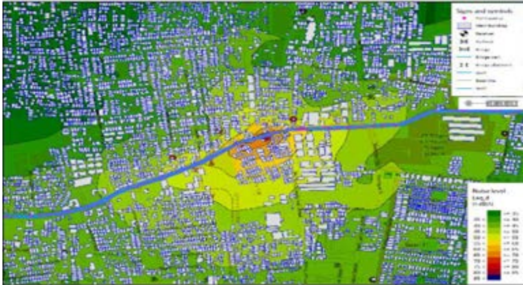
Figure 5-4: Narayanan E-Techno School- After Mitigation - Noise contour maps for Construction phase
