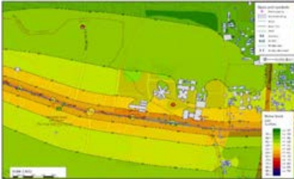
Figure 5-44: Day time Noise contour map for Operation phase (Chennai Bypass Crossing – Ramchandra Hospital).
