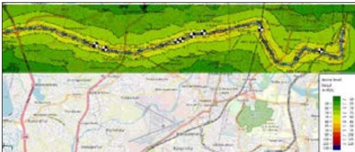
Figure 5-12: Construction – Piling operations – Overall- with Mitigation (wall)
