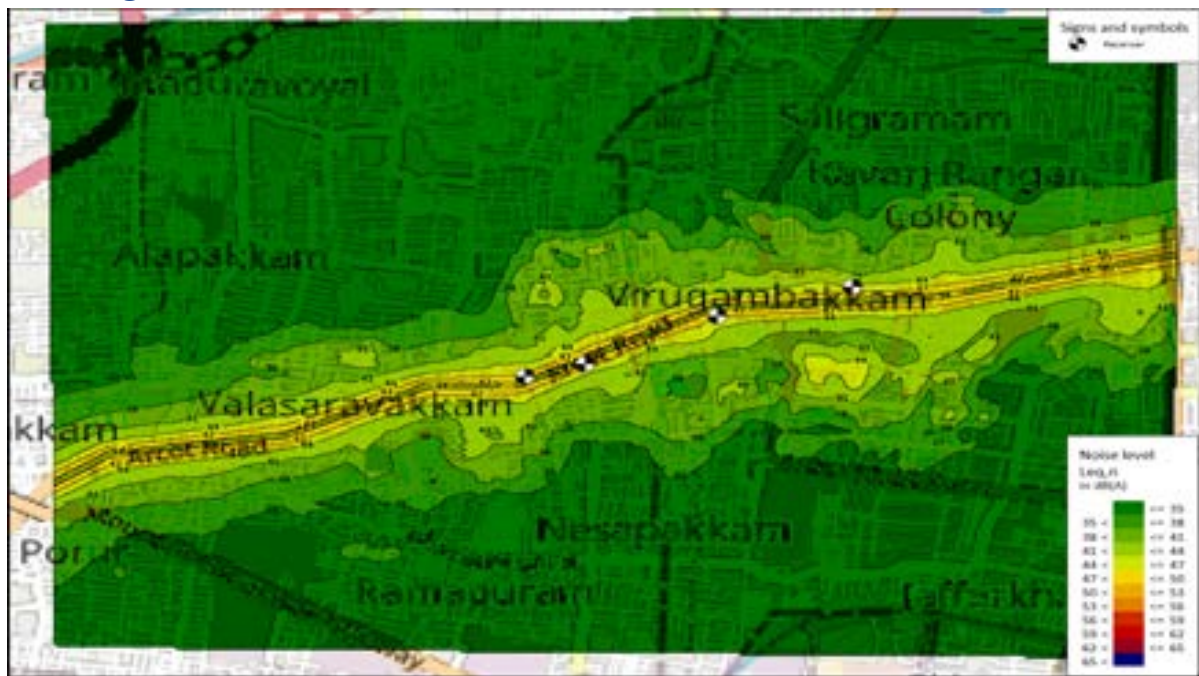
Figure 5-55: Operation Noise at Receiver Location HR-3, 4, 5 & 6 – Night Time- No Mitigation
