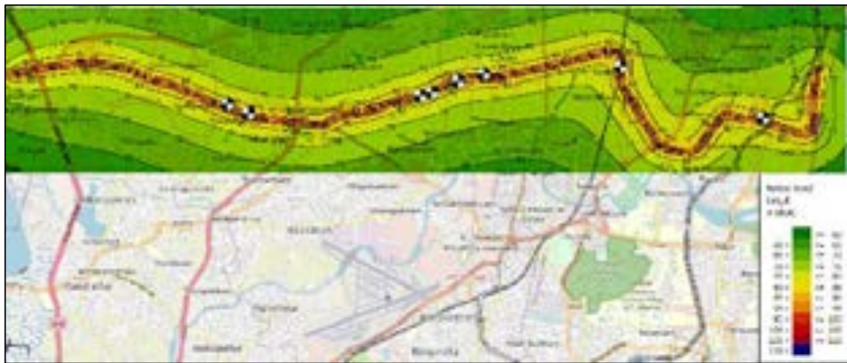
Figure 5-12: Construction – Piling operations – Overall- with Mitigation (wall)
