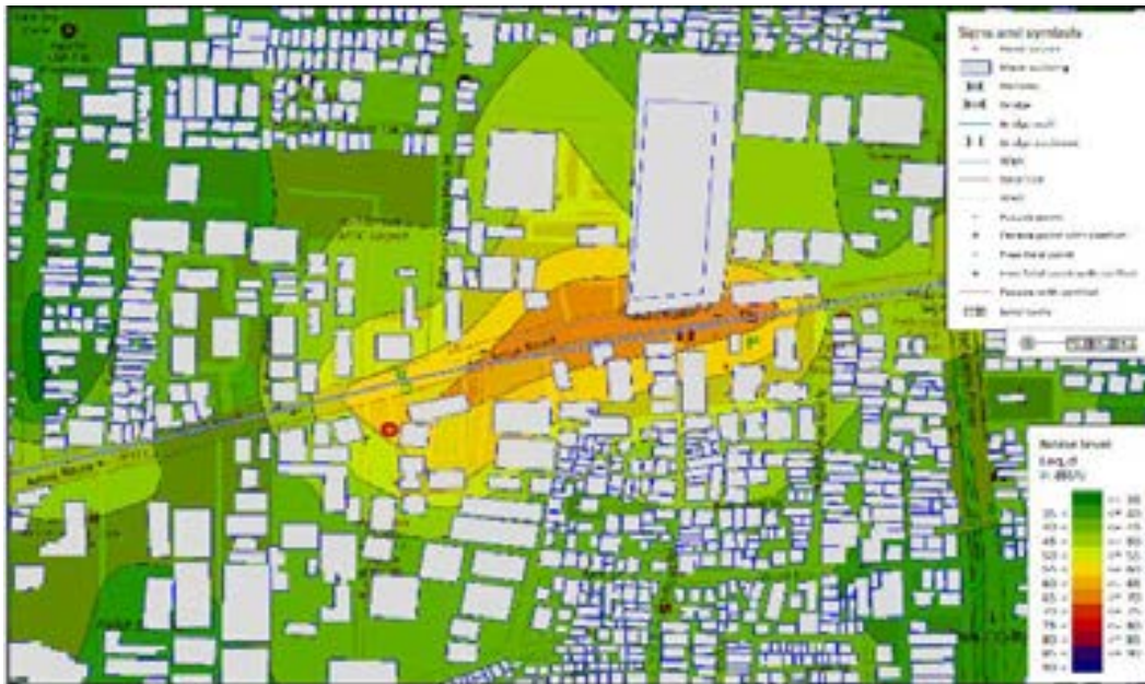
Figure 5-2: Vijaya Hospital - After Mitigation - Noise contour maps for Construction phase.
