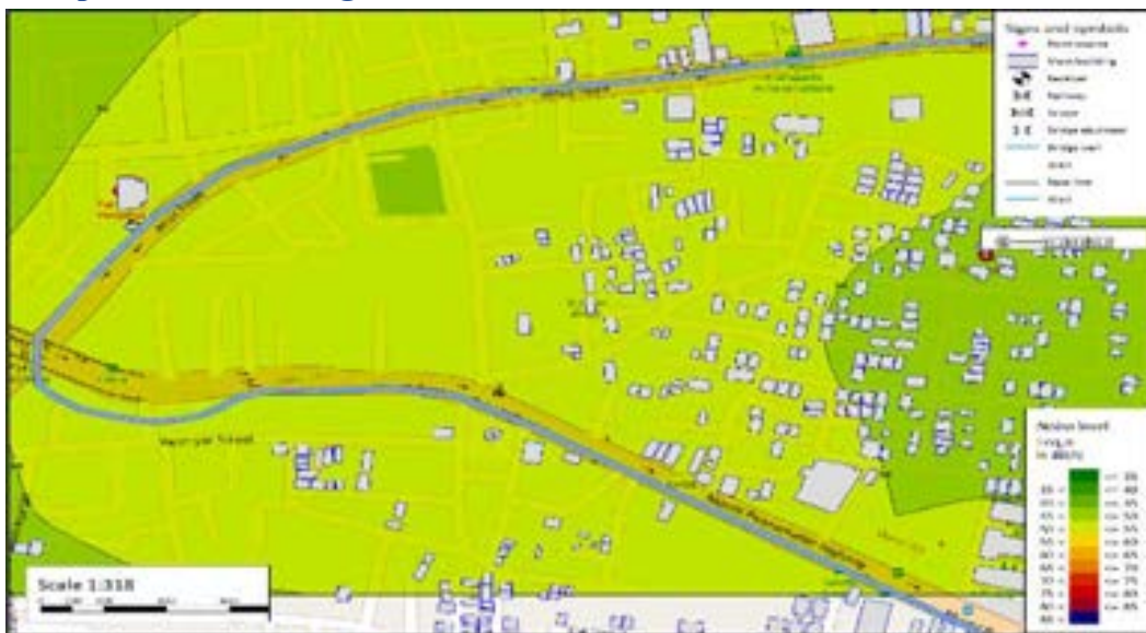
Figure 5-43: Poonamallee Government Hospital- Night time- Noise contour map for Operation phase after Mitigation
