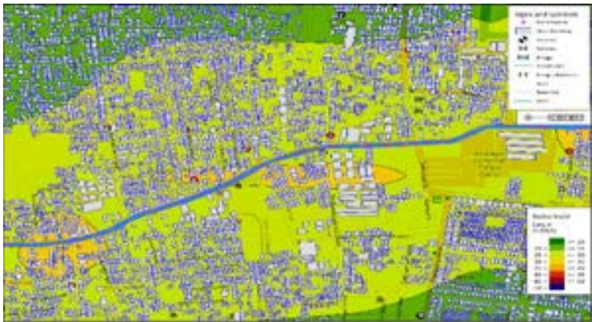
Figure 5-35: Narayanan E-Techno School- Night time- Noise contour map for Operation phase after Mitigation
