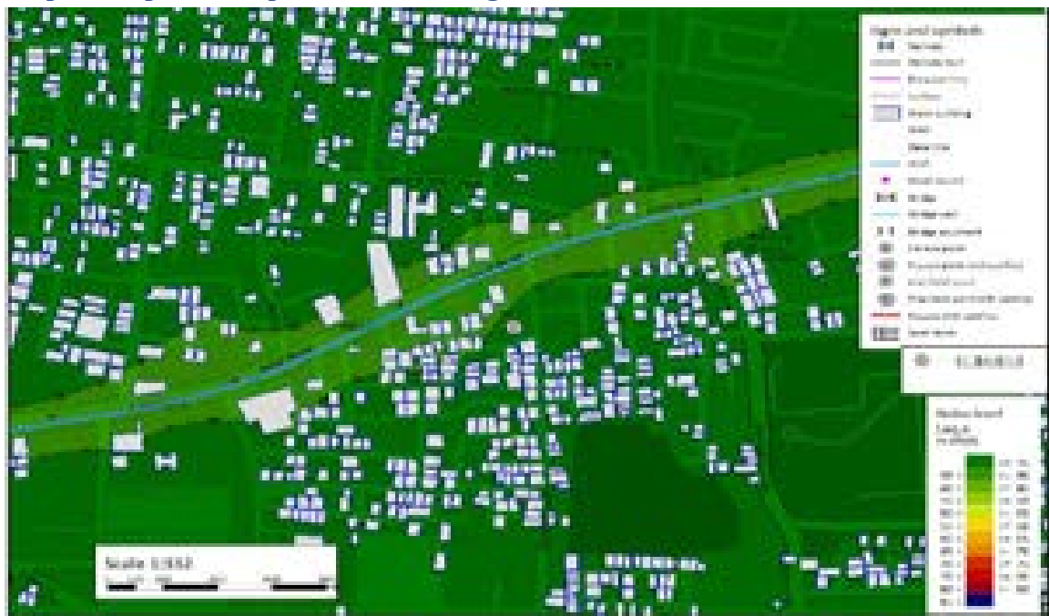
Figure 5-39: The Holy Cross Matric Hr.Sec.School- Night time- Noise contour map for Operation phase after Mitigation
