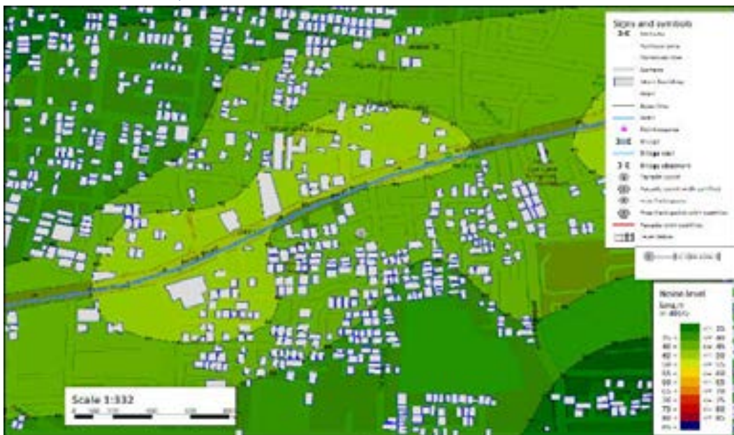
Figure 5-37: Night time Noise contour map for Operation phase (Valasaravakkam – Karambakkam).
