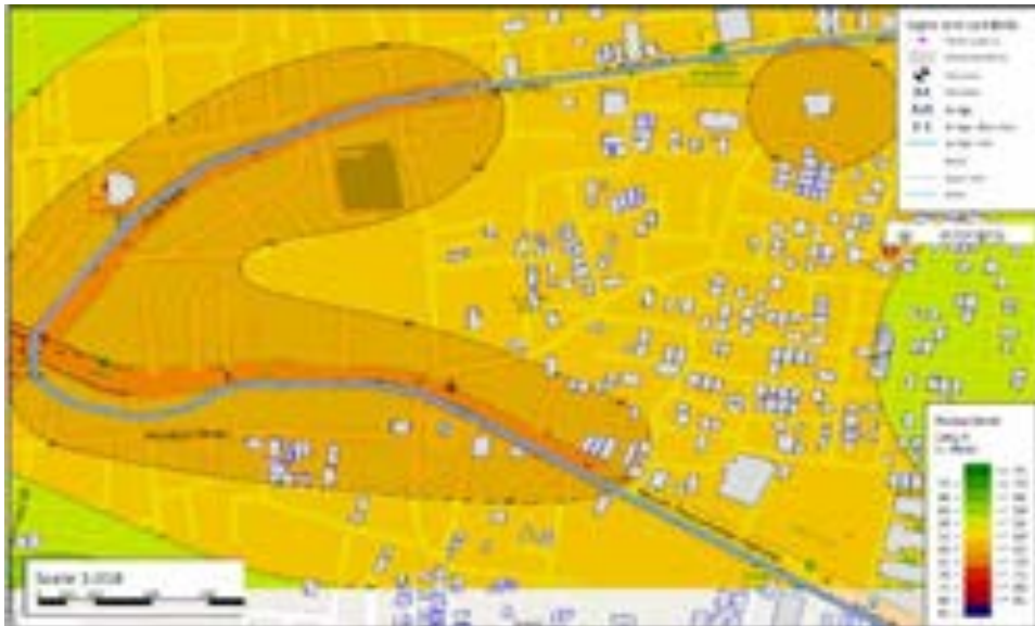
Figure 5-41: Night time Noise contour map for Operation phase (Mullai Thottam – Poonamallee Bus Terminus).
