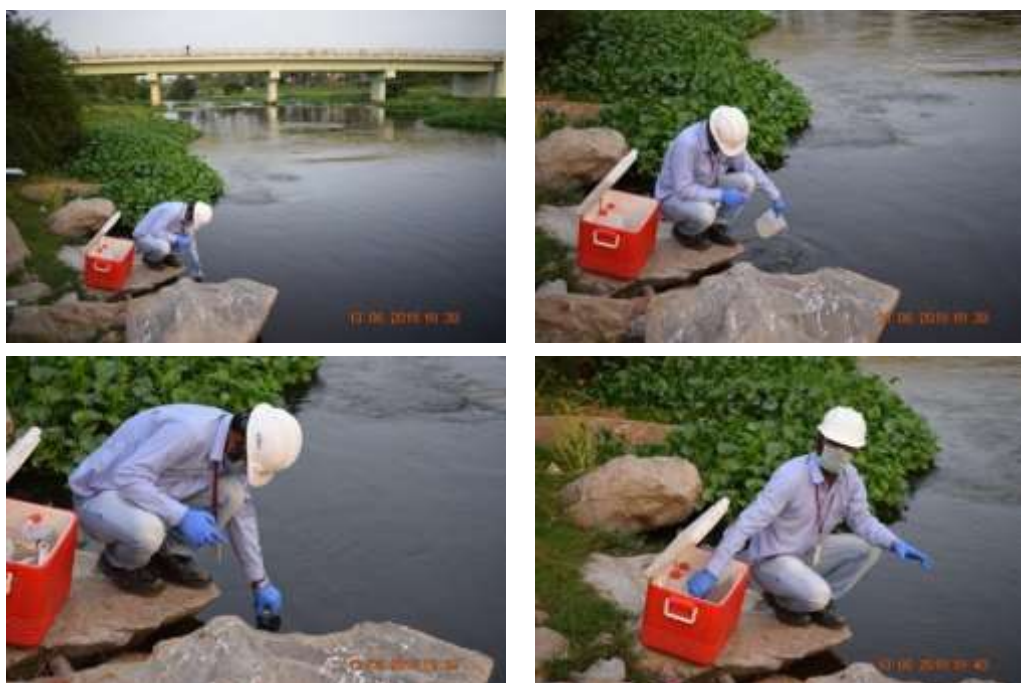
Figure: 3.17: Photograph Showing Water Quality Sampling at Project Site
