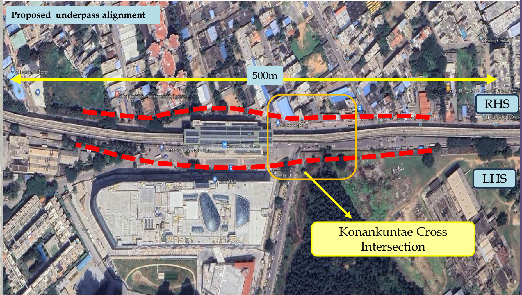
Figure 221: Map Showing the proposed flyover / Underpass Alignment
