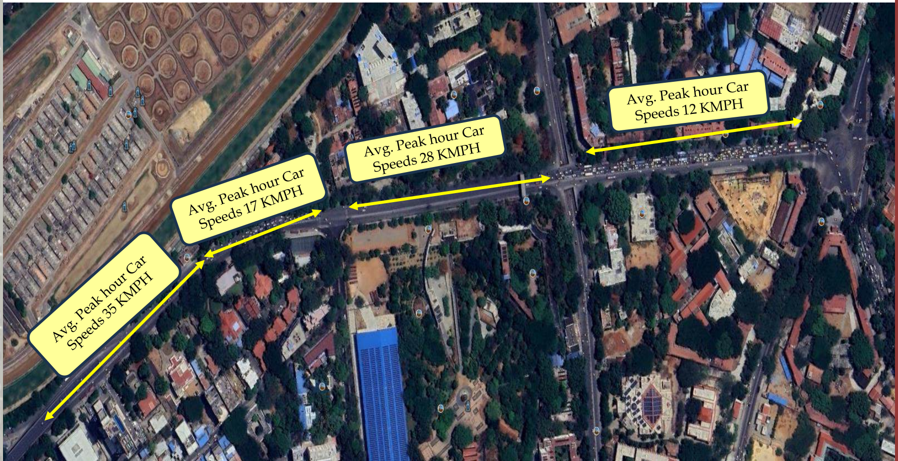
Figure 247. Average Peak Hour car speed from Anand Rao Flyover to K.R. Circle
