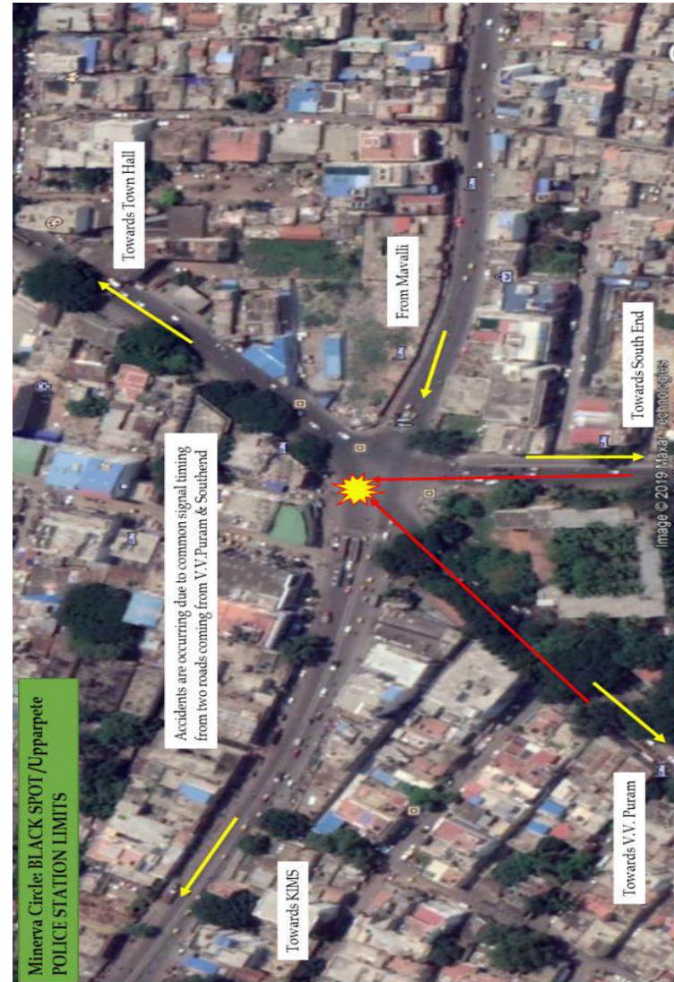
Figure 172. Identification of Black Spot at Minerva Circle
