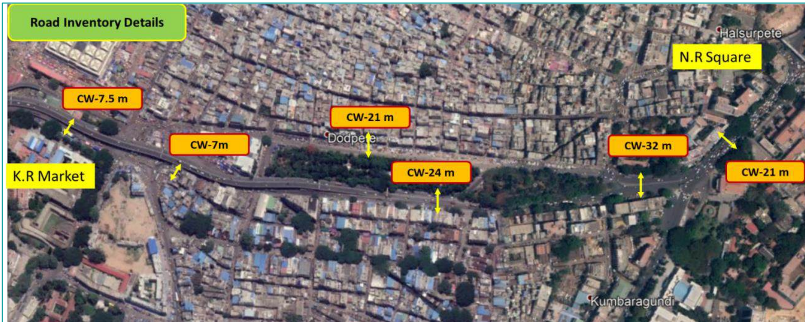
Figure 305. Road Inventory along Mysore Road
