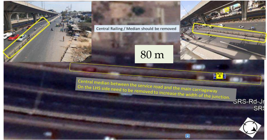
Figure 73. Recommendations for Issues at SRS Junction.
