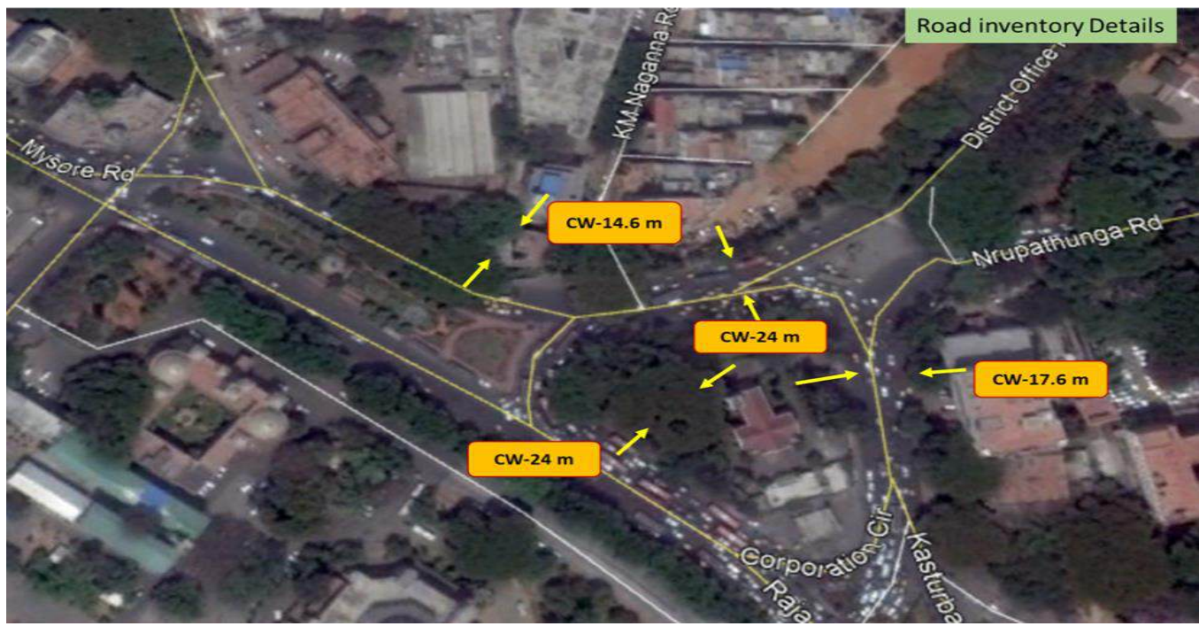
Figure 163: The Road Inventory Survey for Jayachamaraja wodayar road
