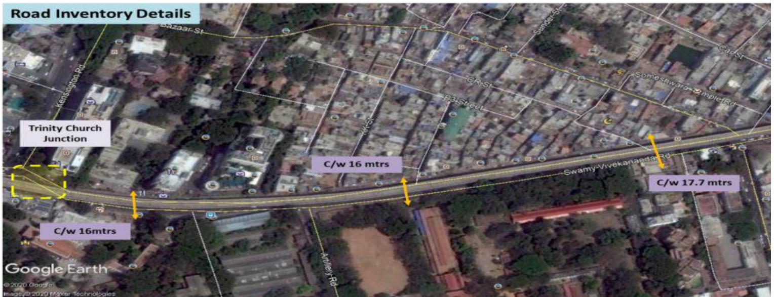
Figure 108 Road Inventory Survey Details
