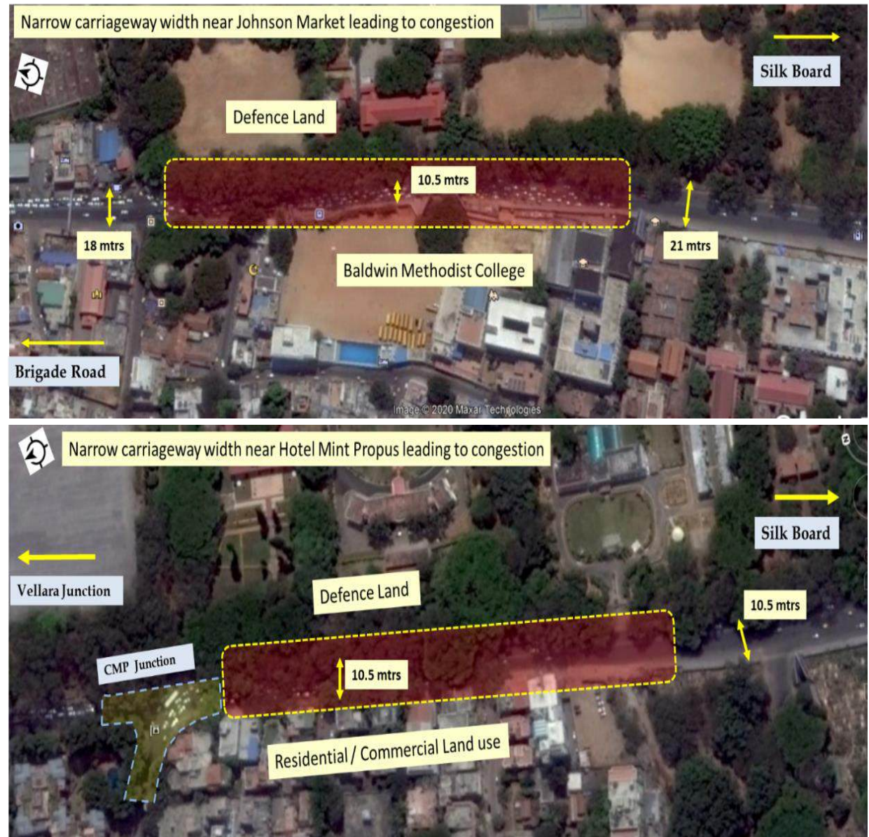
Figure 274. Issues near Johnson market junction
