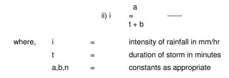
The available data on 'i' and 't' are plotted and the values of the intensity (i) can be determined for any given time of consideration, ( $t_c$ ).
