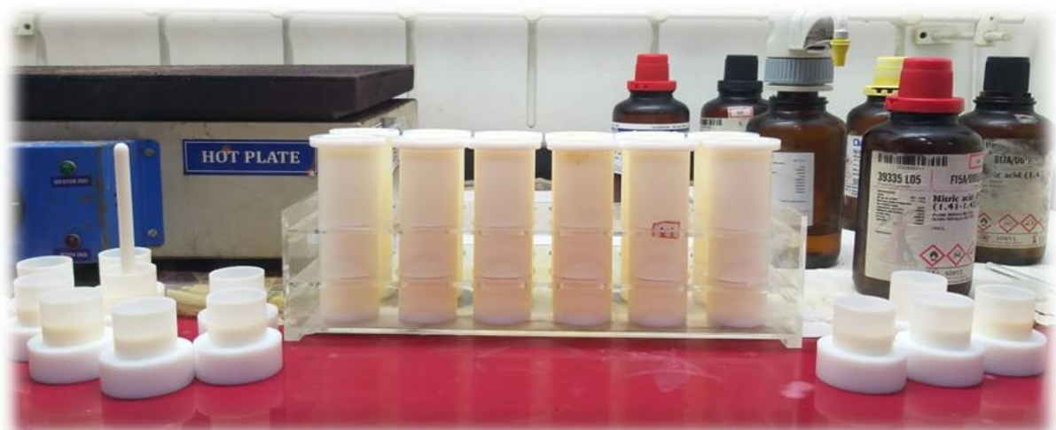
Photo 13. Digested vegetable samples kept for cooling
