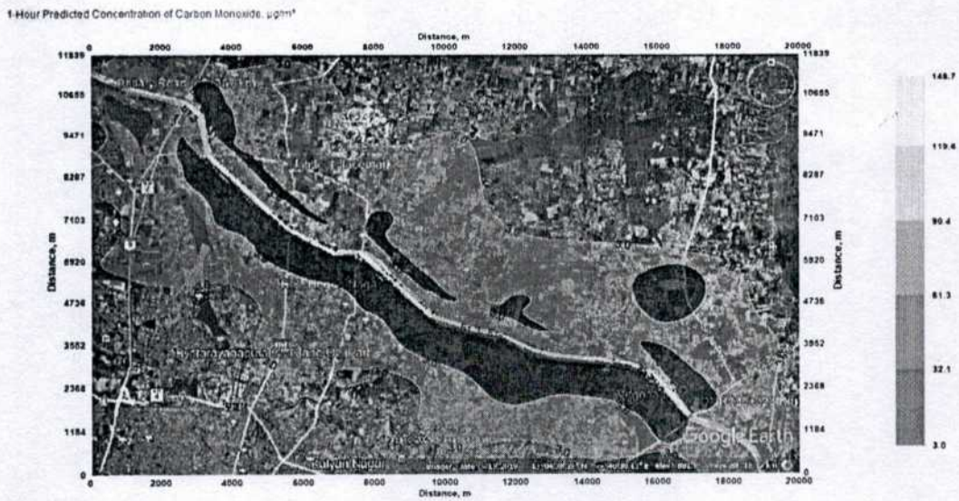
Fig 11: Isopleth showing predicted concentration of CO in Section 2 of PRR alignment during the year 2032 (Operation phase)
