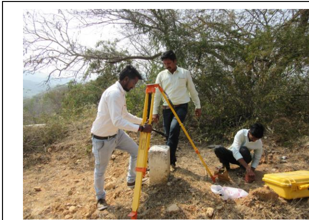
Fig. 4.5: DGPS survey at Bridge location
