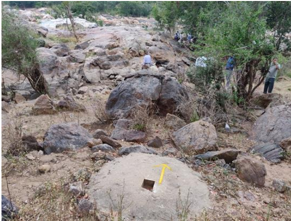
Fig. 1.7: Borehole location along the Dam central line
