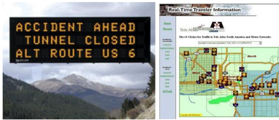
Figure 6-56 Examples of Advanced Traffic Management Systems
