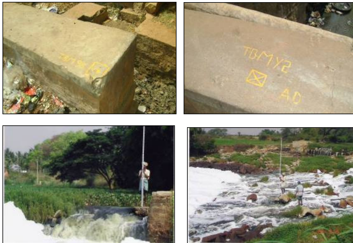
TBMs established at different locations and drain reaches,
