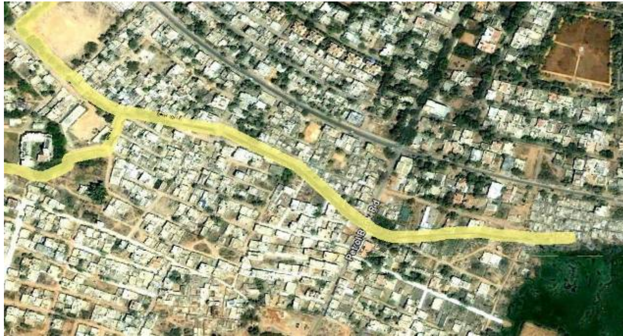
Identification of SWD and demarcation of drainage corridor using Satellite Images
